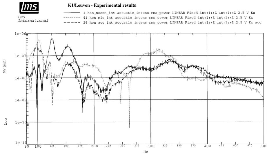
Figure 2. Acoustic intensity radiated by the actuator in the case where only the actuator is mounted in the transmission wall. Solid : without control ; dashed : control using 4 accelerometers as error sensors ; dotted : control with 2 error microphones.
