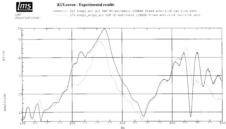
Figure 7. Control voltage sent to the actuator in configuration A. Solid : control with 2 error microphones ; dotted : control using 4 accelerometers on the passive plate as error sensors.
