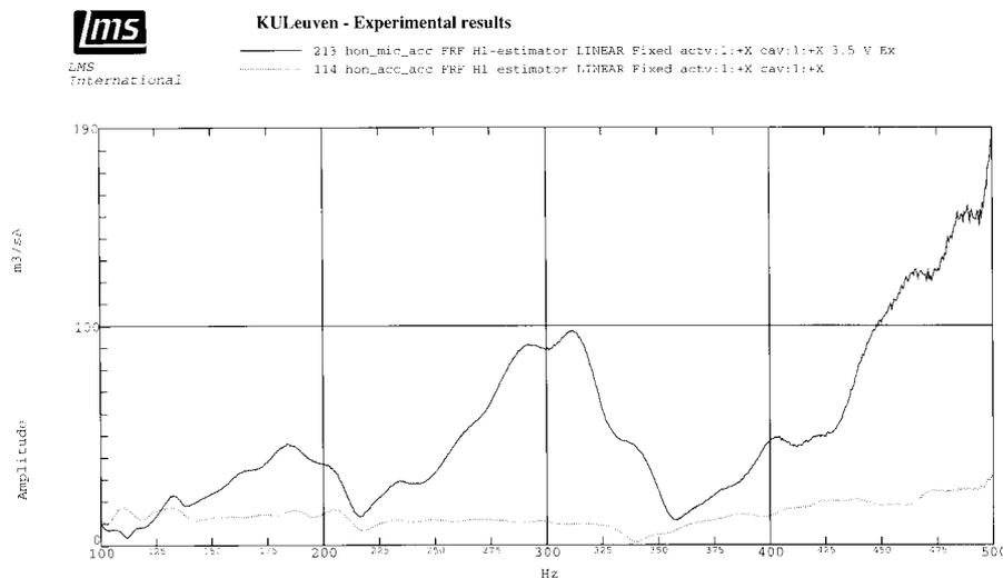
Figure 4. Control voltage sent to the actuator in the case where only the actuator is mounted in the transmission wall. Solid : control with 2 error microphones ; dotted : control using 4 accelerometers as error sensors.
