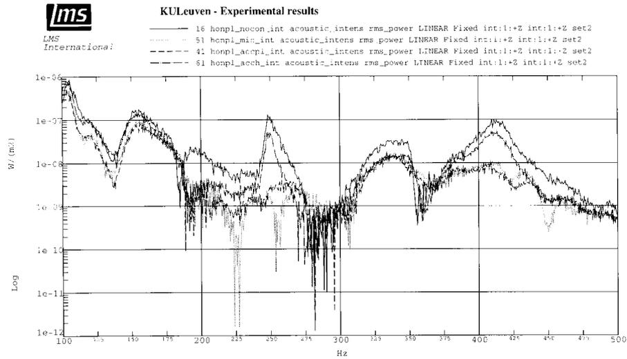
Figure 5. Acoustic intensity radiated by the panel in configuration A. Solid : without control ; dashed : control using accelerometers on the passive plate as error sensors ; dash-dot : control using accelerometers on the actuator as error sensors ; dotted : control with 2 error microphones.
