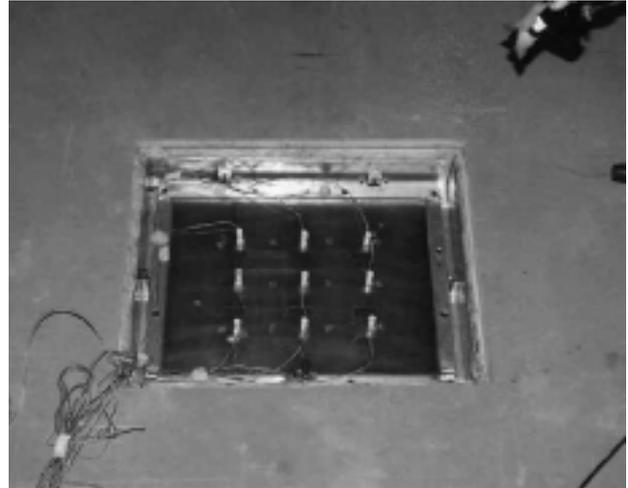
Figure 1b. View on the control actuator mounted in a frame in the transmission wall. The frame allows to mount a steel plate above or below the actuator. The vibration level of the actuator is measured by means of 9 accelerometers.
