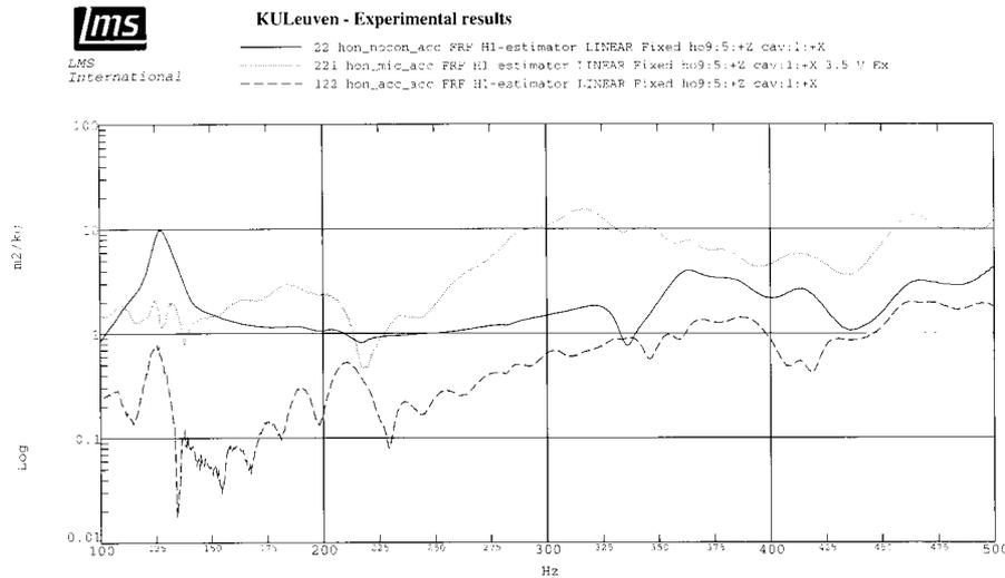
Figure 3. Vibration level measured in the centre of the actuator in the case where only the actuator is mounted in the transmission wall. Solid : without control ; dashed : control using 4 accelerometers as error sensors ; dotted : control with 2 error microphones.
