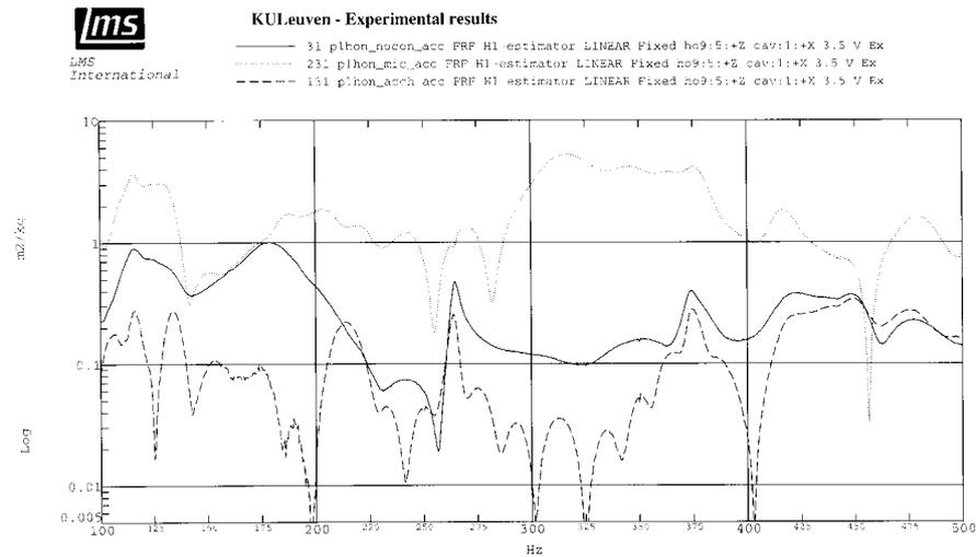
Figure 9. Vibration level measured in the centre of the actuator in configuration B. Solid : without control ; dashed : control using 4 accelerometers on the passive plate as error sensors ; dotted : control with 2 error microphones.
