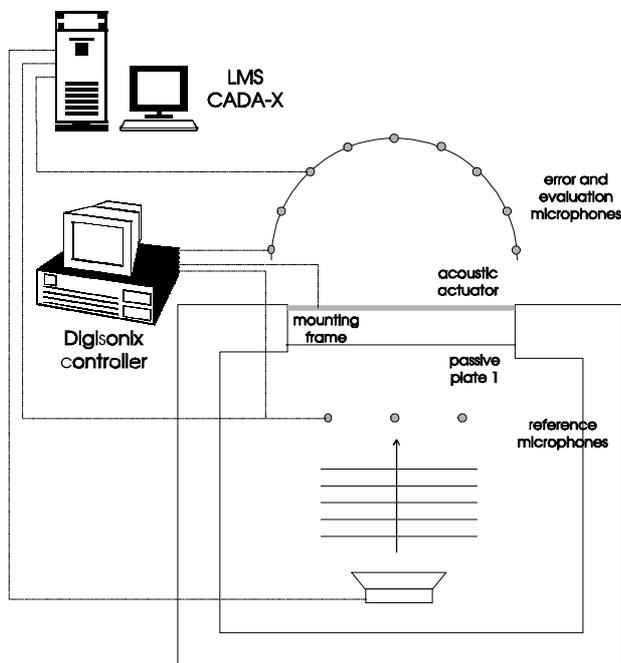
Figure 1a. Schematic overview of the test set-up.
