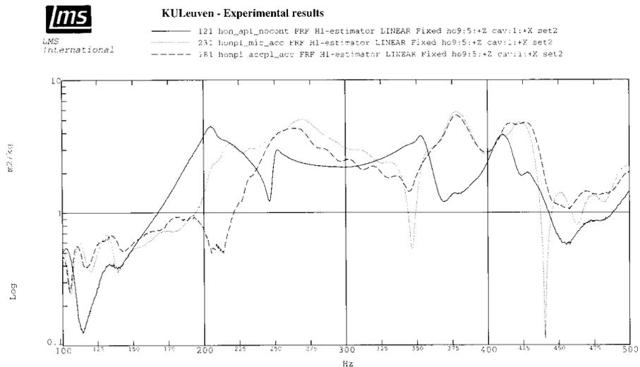
Figure 6. Vibration level measured in the centre of the actuator in configuration A. Solid : without control ; dashed : control using 4 accelerometers on the passive plate as error sensors ; dotted : control with 2 error microphones.
