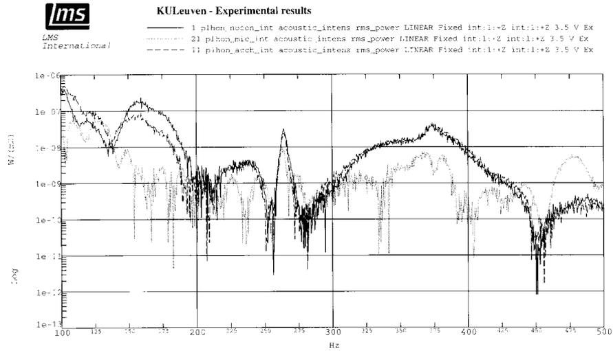
Figure 8. Acoustic intensity radiated by the panel in configuration B. Solid : without control ; dashed : control using accelerometers on the passive plate as error sensors ; dash-dot : control using accelerometers on the actuator as error sensors ; dotted : control with 2 error microphones.
