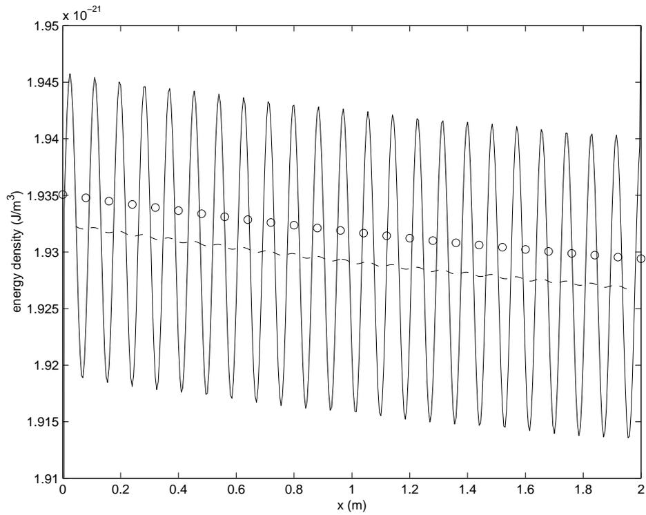
Figure 4: 1D acoustic tube with fluid (air) damping and absorption boundary conditions ( $a = 0.4$ )
