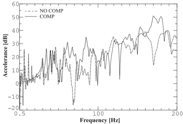
**Figure 3:** Coupled FRFs obtained by FBS using synthesized FRFs with and without dynamic FRF compensation (vertical excitation on the subframe and vertical response on the body roof)
