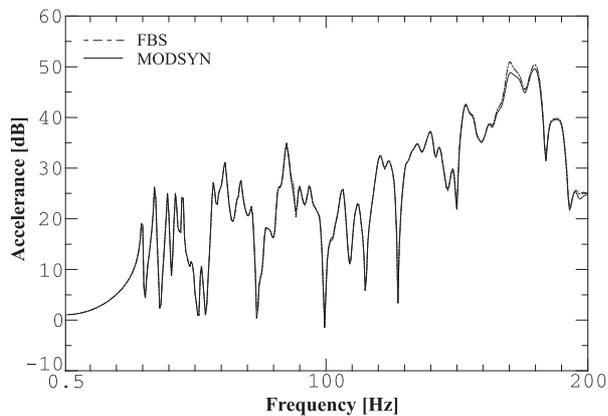
**Figure 4:** Coupled FRFs obtained by FBS and modal synthesis for normal modes with compensation by residual modes (vertical excitation on the subframe and vertical response on the body roof)
