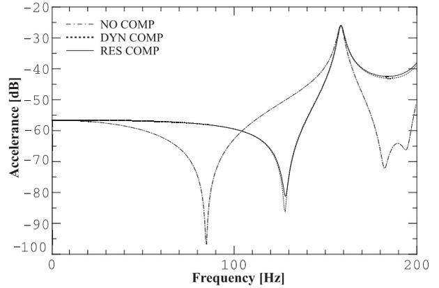
**Figure 2:** Synthesized FRFs of the subframe with compensation (dynamic FRF compensation and compensation by residual modes) and without compensation (rotational excitation and rotational response dof)
