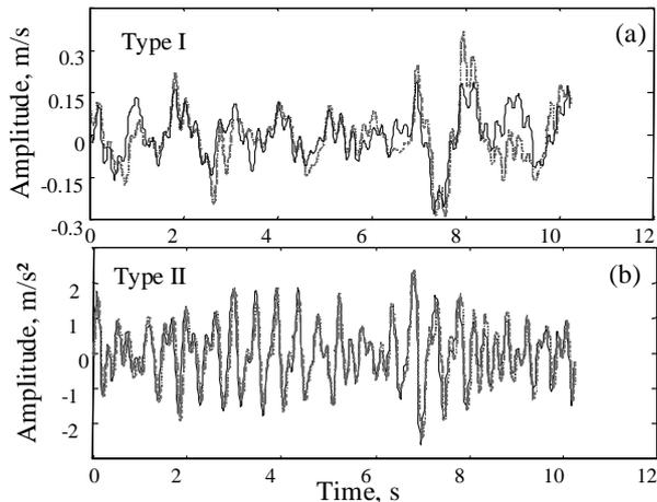
Figure 5: (a) Comparison between the amplitudes of the models outcome (6-5-1) (full line) and the measured horizontal velocity of the boom tip (dotted line); (b) comparison between the amplitudes of the models outcome (6-6-1) (full line) and the measured vertical accelerations of the boom tip (dotted line).
