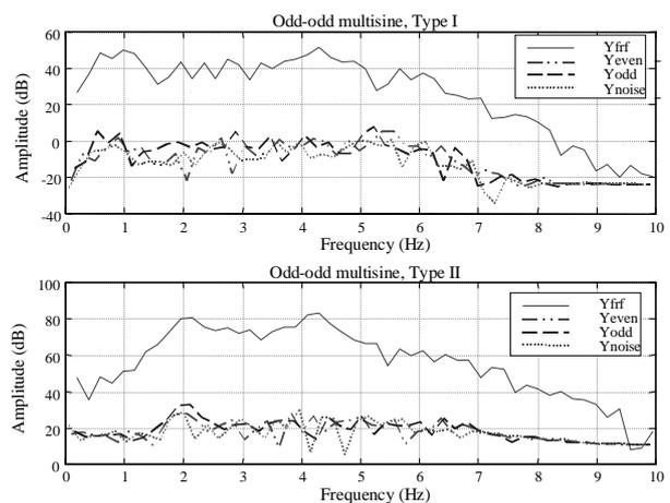
Figure 3: Detection of non-linear distortions at the output of the boom tip for horizontal and vertical direction.  $Y_{fir}$ : linear + odd non-linear contributions,  $Y_{even}$ : even non-linear contributions,  $Y_{odd}$ : odd non-linear contributions,  $Y_{noise}$ : noise level.
