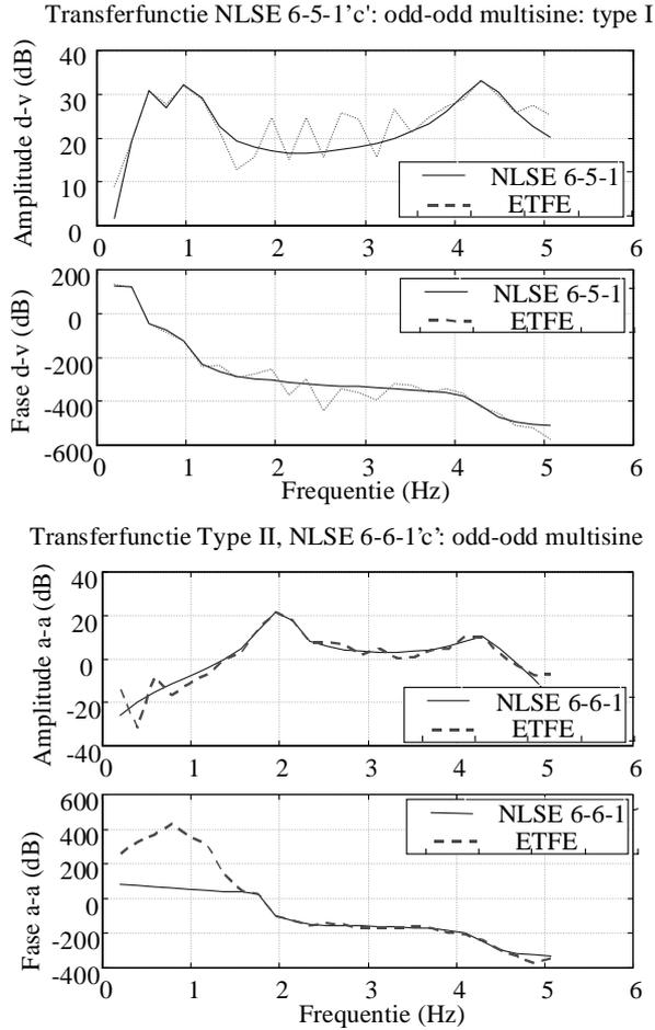
Figure 4: Comparisons between the amplitudes and phases of the transfer function estimates (full line) and the measured frequency response function (dotted line) for longitudinal and vertical direction respectively; excitation with odd-odd multisine.
