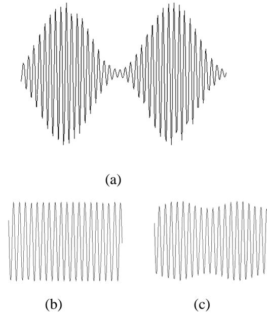
**Fig. 10.** Schematically shown principle of the method: (a) - the strong (pump) modulated wave; (b) - the excitation signal for the weak probe wave; (c) - appearance of the probe-wave modulation due to the material nonlinearity.
