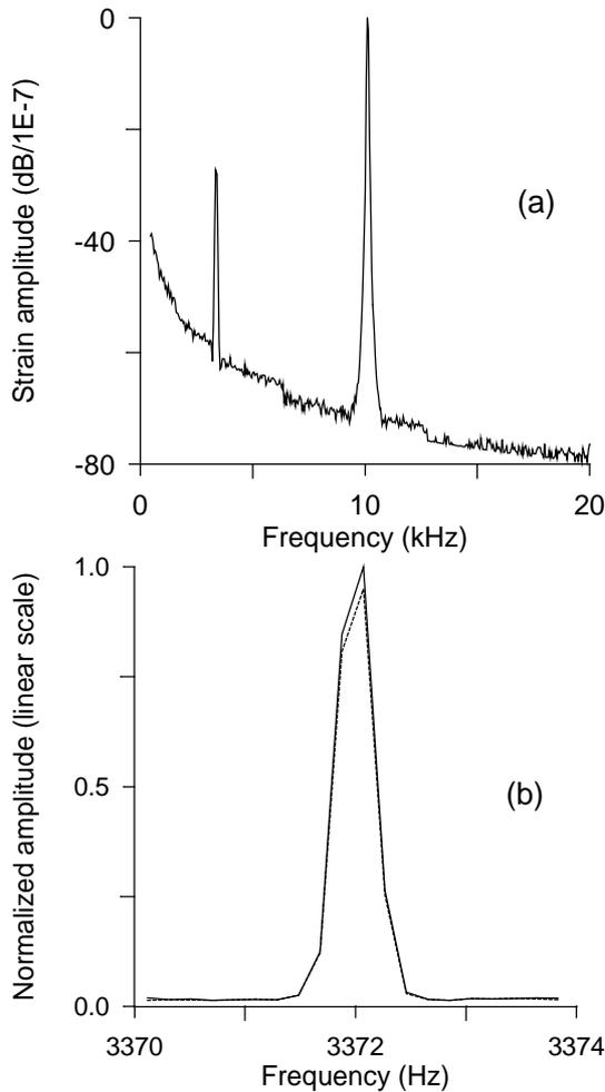
**Fig.9** Suppression of the probe wave under the action of the pump wave due to the dissipative nonlinearity of the material.
