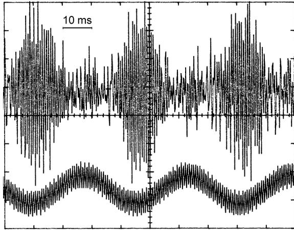
**Fig.4.** Temporal record of the vibration in the damaged sample at a strong modulation. The lower record is the excited superposition of the LF and HF signals measured by accelerometer 7. The upper record is the modulated HF signal received by accelerometer 8 (the LF signal is filtered out).
