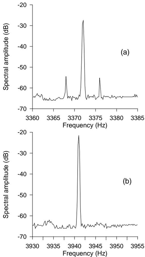
**Fig. 10.** An example of the modulation spectrum obtained in the microinhomogeneous copper rod (a) and the similar spectrum without signs of modulation obtained at similar conditions in the reference homogeneous rod made of glass (b).
