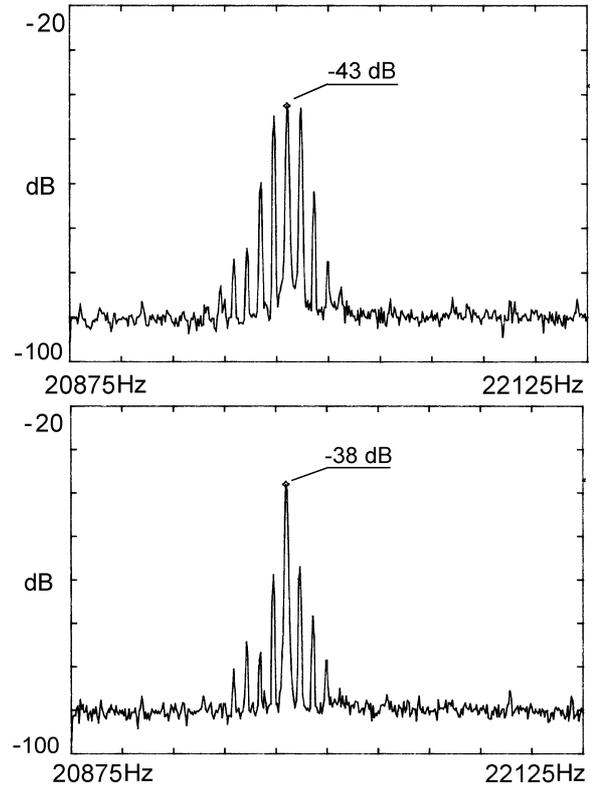
**Fig. 7.** The modulation spectrum for the damaged sample before (upper record) and after (lower record) the introduction of additional losses by sticking the rubber strips.
