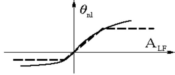
**Fig.5.** Schematically shown amplitude dependence of the nonlinear losses (the solid curve) and its approximation by a piece-wise function (the dashed curve).
