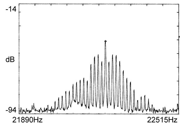
**Fig.3.** Example of a very rich spectrum with strong higher-order side-lobes in the damaged sample.
