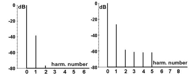
**Fig.6.** Example of the simulation of the modulation spectra at lower (left) and higher (right) LF vibration amplitudes.
