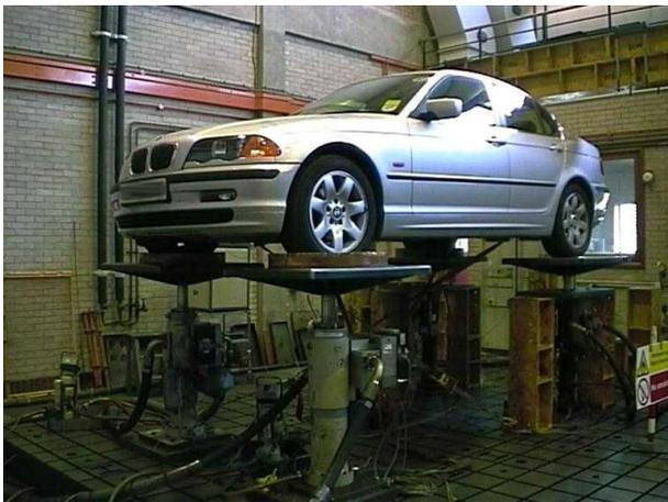
Figure 1: Experimental set-up: industrial 4 poster test rig
