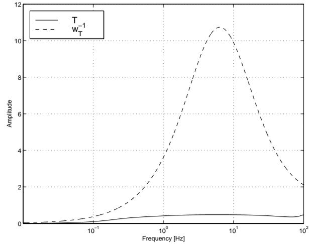
Figure 7: Complementary sensitivity function  $T$  and inverse of weighting function  $w_T$
