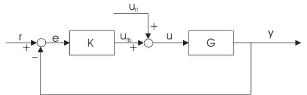
Figure 3: Used control scheme: off-line calculated feed-forward ( $u_{ff}$ ) + real-time feedback ( $u_{fb}$ )
