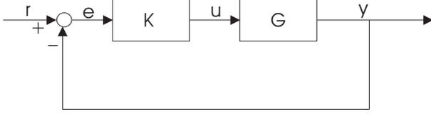
Figure 2: 1 DOF feedback control scheme
