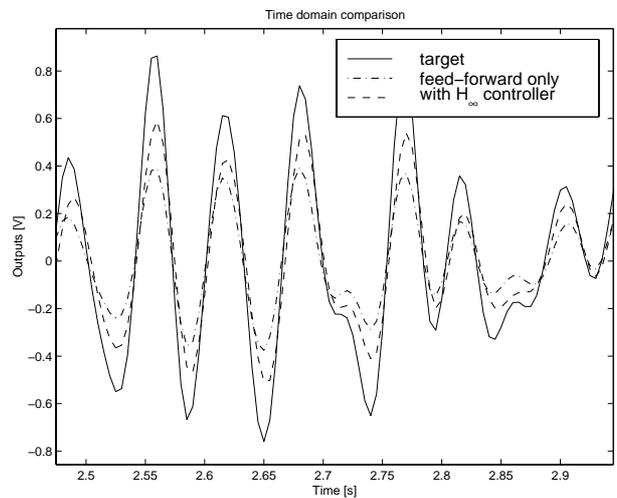
Figure 8: Comparison of target signal with signals measured when using feed-forward only on the one hand and with the  $\mathcal{H}_\infty$  controller on the other hand
