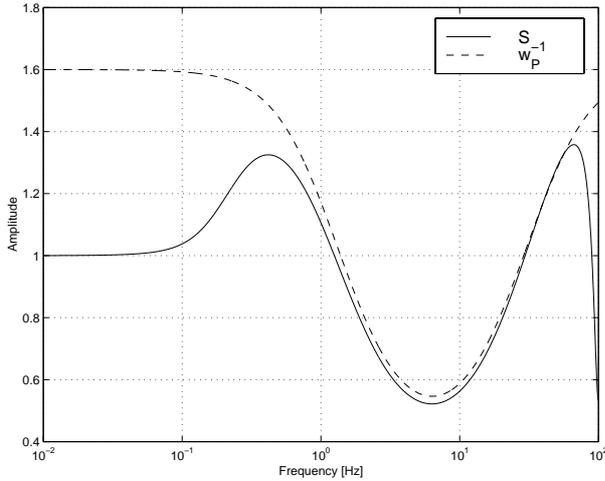
Figure 6: Sensitivity function  $S$  and inverse of weighting function  $w_P$
