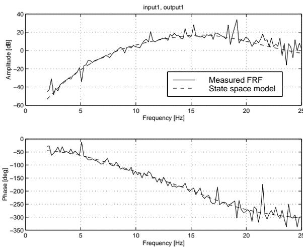
Figure 4: Comparison between non-parametric FRF model with transfer function from state space model
