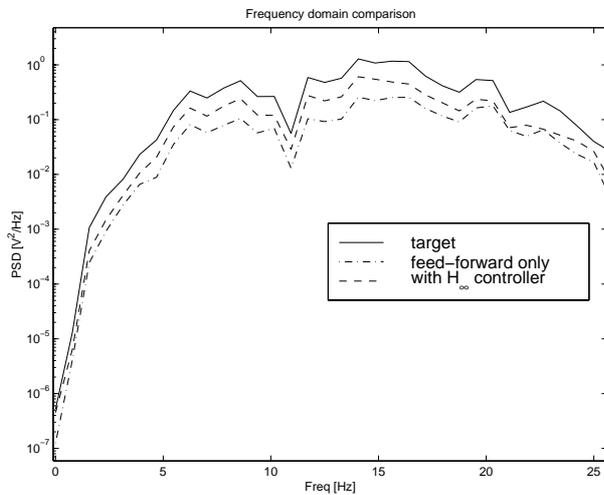
Figure 9: PSD comparison of target signal with signals measured when using feed-forward only on the one hand and with the  $\mathcal{H}_\infty$  controller on the other hand
