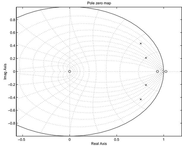
Figure 5: Poles and zeros of the identified state space model
