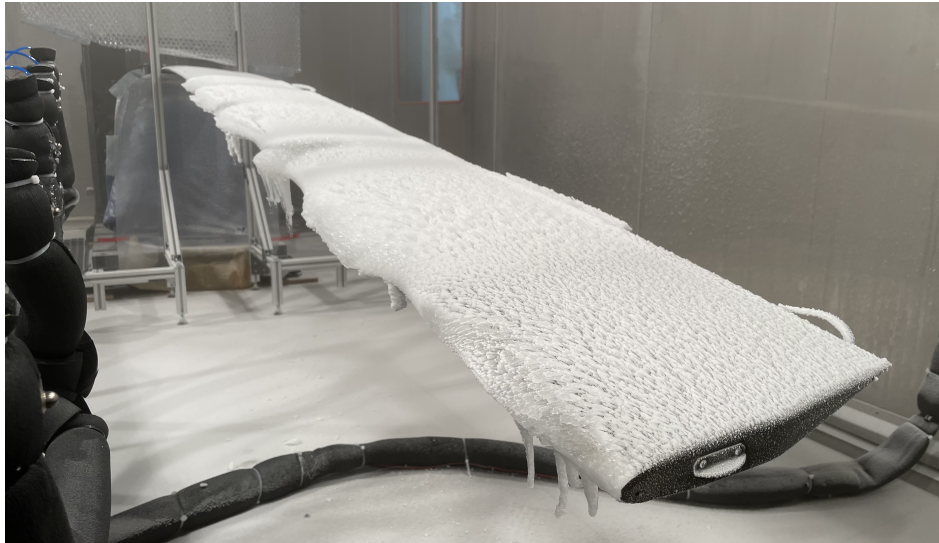
Figure 7: Helicopter blade during ice accumulation tests.
