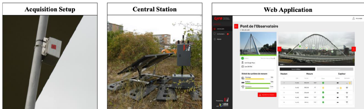
Figure 2: Overview of the LYRA monitoring solution showing a wireless sensor mounted on a cable (left), the central station with its solar panel (middle) and the web application (right).
