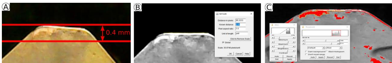
Figure 6: (a) initial picture (b) 8 bit black and white picture with a horizontal edge (c) highlighting of the degradation area.
