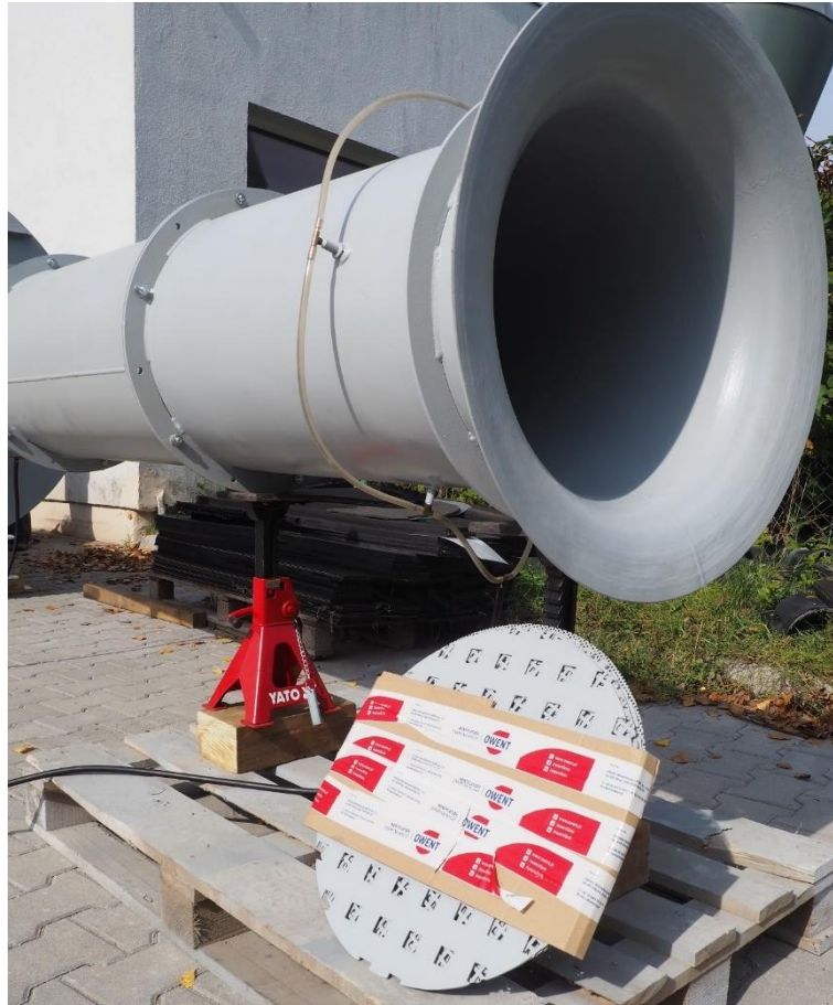
Figure 7. Start of the inlet nozzle for the fan together with the special test
