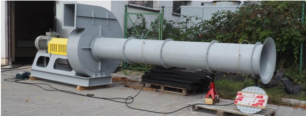
Figure 4. Test stand to test the prototype of the centrifugal fan in accordance with standard EN ISO 5801
