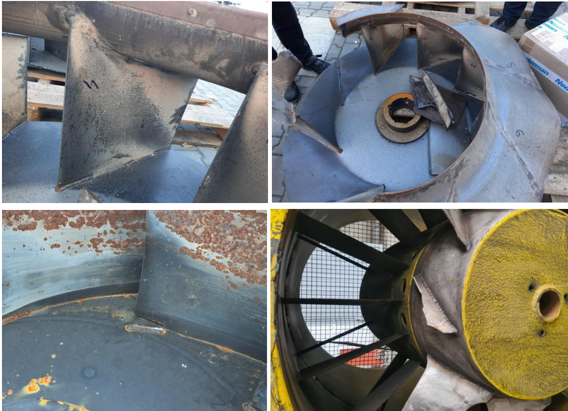
Figure 1. Fatigue failures of industrial fans
