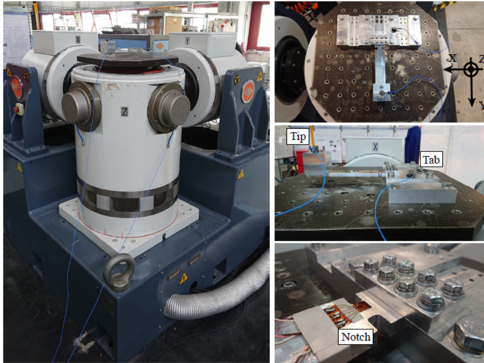
Figure 1: Experimental setup: 3-DoF shaker table Dongling 3ES-10-HF-500(left); top views of the specimen (right-top); side view of the specimen (right-middle); detail of strain gauge rosette applied on the notch (right-bottom).
