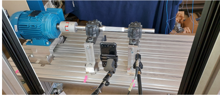
Figure 9: A picture of the test rig with additional DC lighting and a smartphone and microphone mounted on a tripod.
