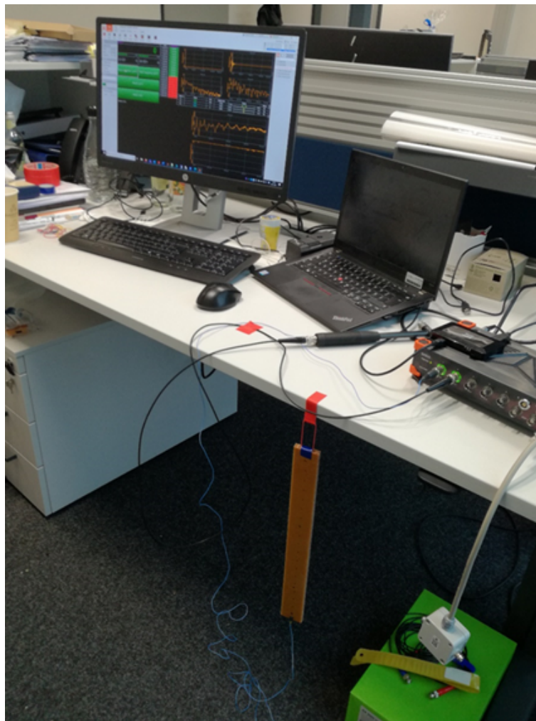
Figure 3: Free-hung sandwich beam and a simplified impact test set-up
