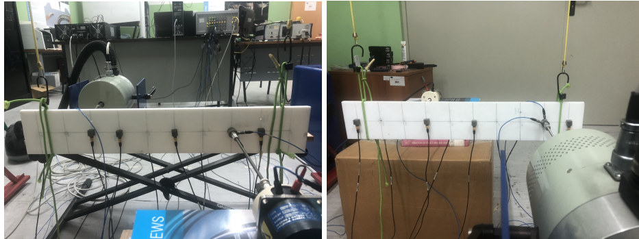
Figure 1: Experimental case study: PTFE beam in free-free boundary conditions. Forces are simulated by two modal shakers attached by stinger.
