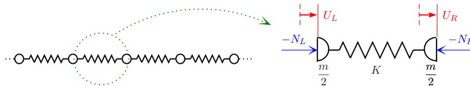
Figure 1: Unit cell of a discretized rod
