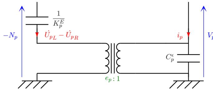
Figure 8: Global model of the piezoelectric element
