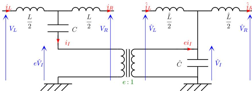
Figure 7: Coupling of two electrical networks
