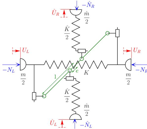
Figure 4: Unit cell for two coupled discretized rods
